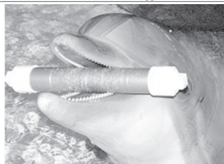
This dolphin is carrying a device that measures the movement of its head as it swims.
