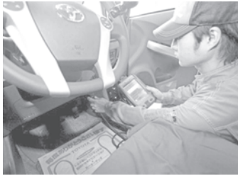
A Toyota mechanic fixes the anti-lock brake (ABS) software on a Prius hybrid vehicle at a dealer's repair shop at Nagoya city in Aichi prefecture, in central Japan, February 2010.—INTERNET
