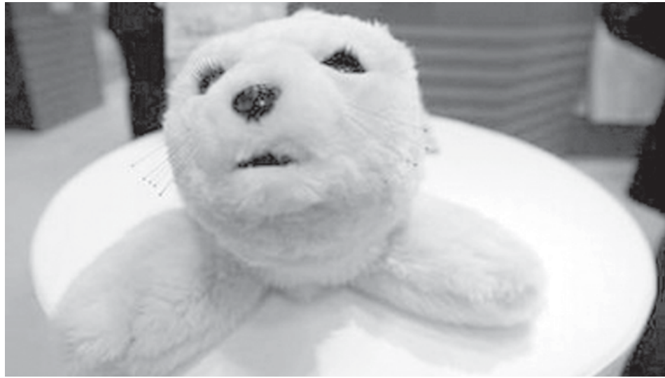
A furry robotic seal called "Palo" is pictured at the International Robot Exhibition in Tokyo on 28 Nov, 2007. The robot seal, which can learn its name and react to touch, is designed to help elderly people avoid loneliness and develop connections with others by interacting and talking to the robot.—INTERNET
