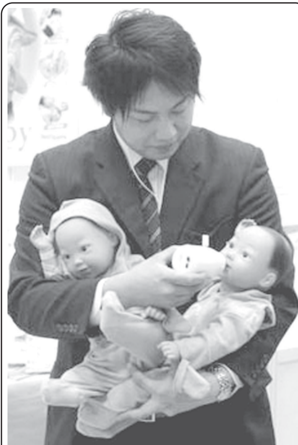
An employee of Yamazaki Educational Systems Co. holds two "My Baby 2" robotic babies at the International Robot Exhibition in Tokyo, on 28 Nov, 2007. The robotic babies are designed to teach parenting skills and require feeding, diaper changes, burping and sleeping and also record data on how their human parents treat them.
