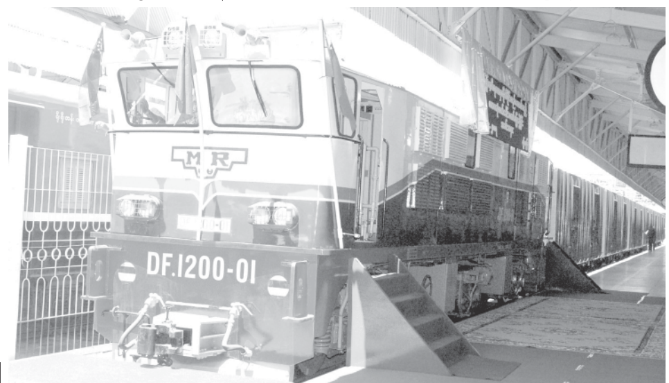
1200-HP diesel engine manufactured by Myanma Railways.
