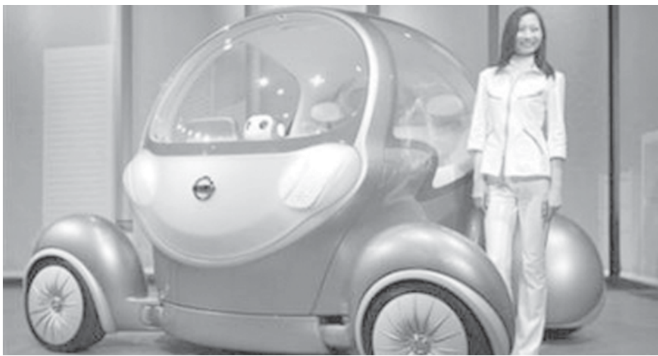
A model poses next to Nissan Motor's concept car 'Pivo 2' during an unveiling for the upcoming Tokyo Motor Show 2007, on 5 Oct, 2007. The concept car, featuring a rotating cabin which can swivel 360 degrees and 90 degrees turning wheels, is powered by compact lithium-ion batteries.— INTERNET
