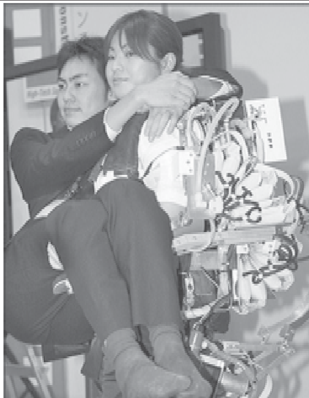
Photo taken on 3 Oct 2007 shows Kanagawa Institute of Technology unveiled a power assisted suit, powered by air pressure for nursing of elderly persons and patients of hospitals, at the Home Care and Rehabilitation Exhibition in Tokyo.
