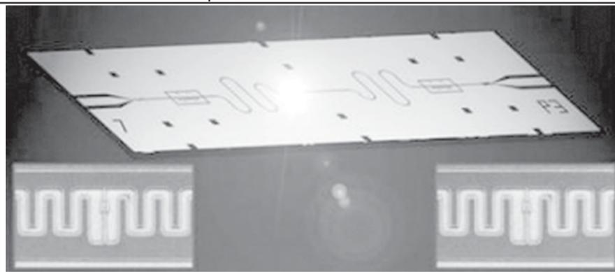
*An image released by Yale University's Schoelkopf Lab on 26 Sept, 2007 shows a microchip that enables quantum information to be shuttled back and forth between two superconducting qubits.*
