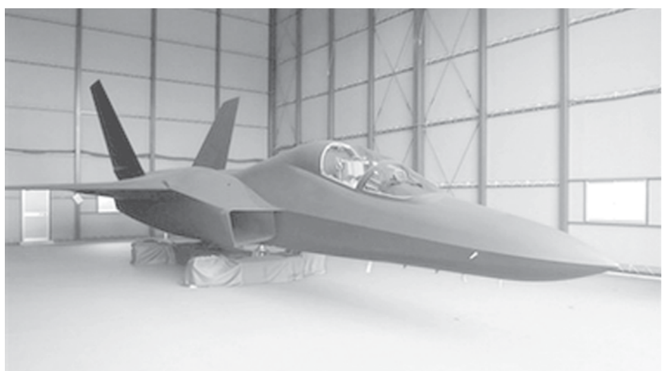
A 14-meter-long (46-foot-long) carbon fibre mock-up of Japan’s next-generation stealth fighter jet sits in Mitsubishi Heavy Industries Ltd’s Komakiminami Factory in Toyoyamacho, Aichi Prefecture (State), central Japan, on 9 Aug, 2007. —INTERNET
