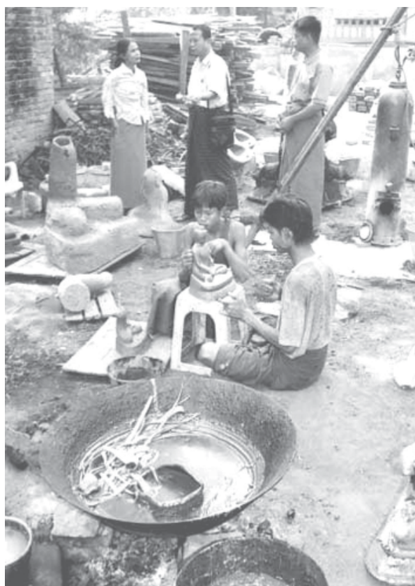
Moulding and waxing section of bronze casting work.
