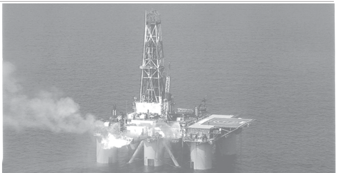
Natural gas being burnt to test its quality at Zawtika-5 Well in M-9 block. — ENERGY
