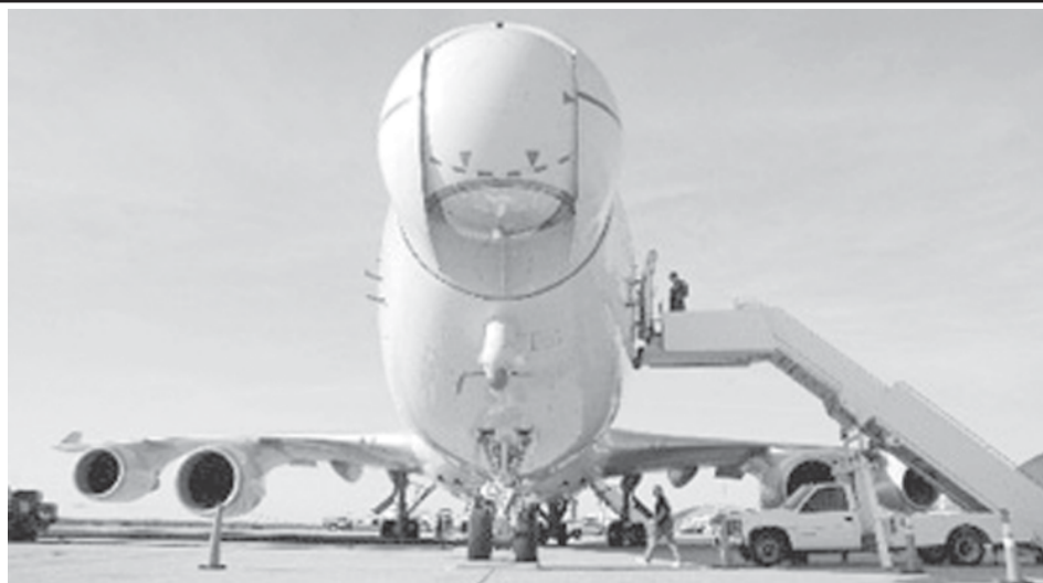
The USAF Airborne Laser aircraft sits on the tarmac at Andrews Air Force Base outside Washington on 21 June, 2007. The modified 747 aircraft uses a high-energy Chemical Oxygen Iodine Laser to generate an energy beam from the aircraft's nose to intercept and destroy a hostile ballistic missile during the boost phase of its trajectory. —XINHUA
