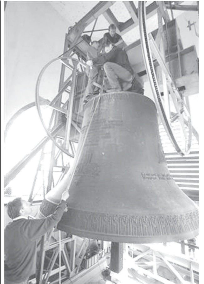
Technicians examine the St Stephens cathedral's bell "Pummerin" to assess possible damage in Vienna on 23 April, 2007. Europe's second largest bell, nicknamed "Pummerin", is one of many famous bells across the continent undergoing a medical check up and examination as part of the "probell" project aimed at determining their life spans and unravelling the secret of the optimum way of chiming. — INTERNET
