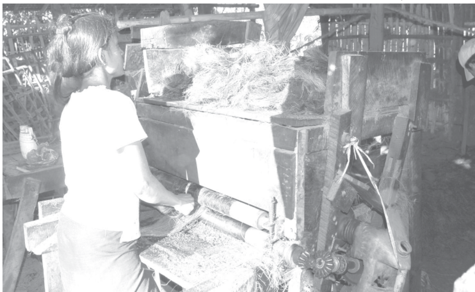
Coconut fibres are twisted into strings with the use of a machine.
