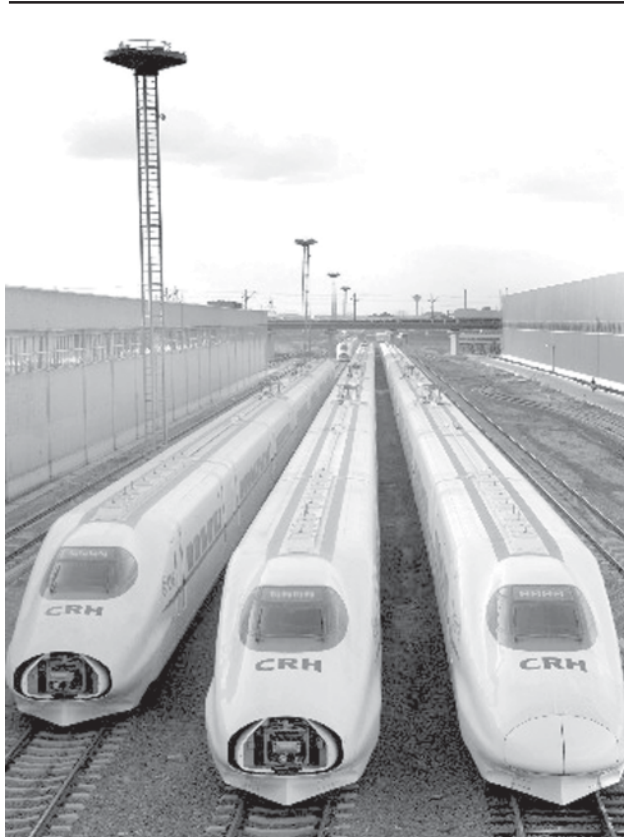
"Hexie" train. China will raise the speed limit for rail traffic for the sixth time on 18 April. A train named "Hexie", one of the China Railway High-speed (CRH) series, will be the focus of the speed increase. The train can run at over 200 kilometres per hour. Each carriage is self-driven and equipped with modern facilities.—XINHUA
