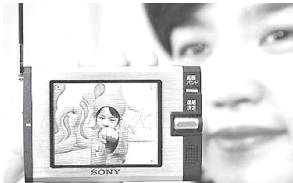
Sony introduces the XDV-100 pocket-size digital TV in Japan. The measurements of the Sony XDV-100 are 98.3x61x15.1mm and the sleek TV weighs only 110g. — XINHUA
