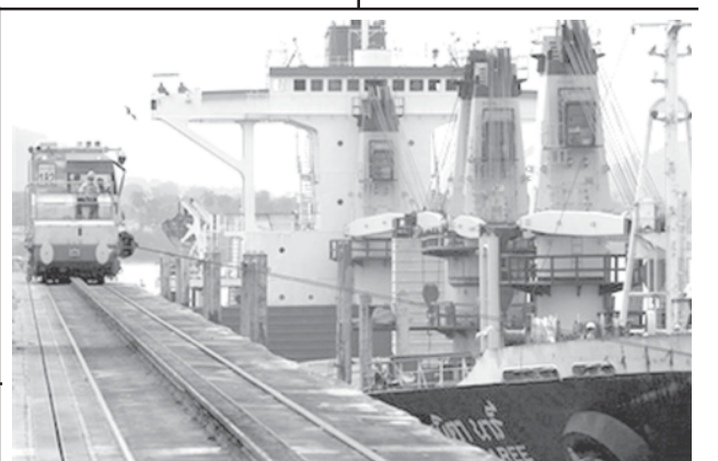
A locomotive guides a cargo ship through the Miraflores Locks in Panama City, on 5 April, 2007. — INTERNET
