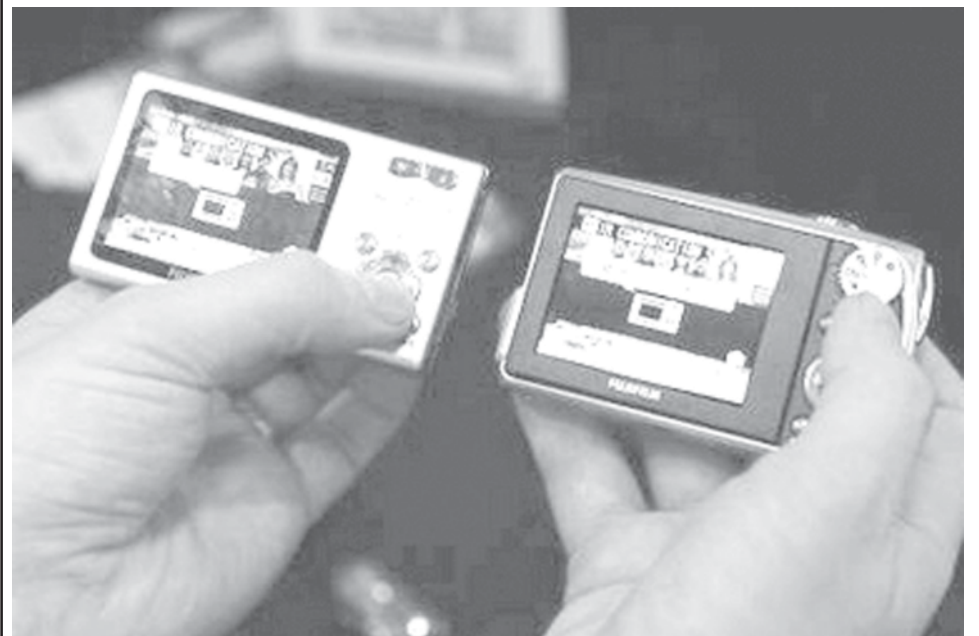
A Fujifilm representative uses IRsimple technology to wirelessly transfer a photo from one camera to another during a preview for the Photo Marketing Association International (PMAI) convention in Las Vegas, Nevada, on 7 March, 2007. The IR (infrared) system can also be used to send a photo to a IRsimple printer. —INTERNET
