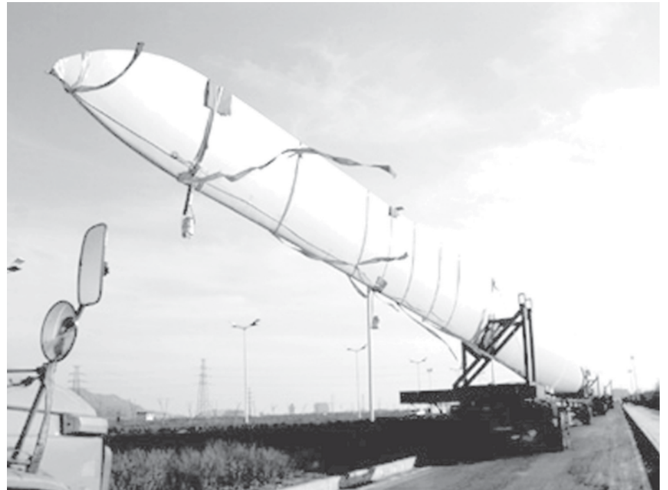
Trucks transport wind turbine blades in Lianyungang City, East China's Jiangsu Province, on 27 Feb, 2007. The 37.5-metre blade is the biggest one on the domestic market.—XINHUA
