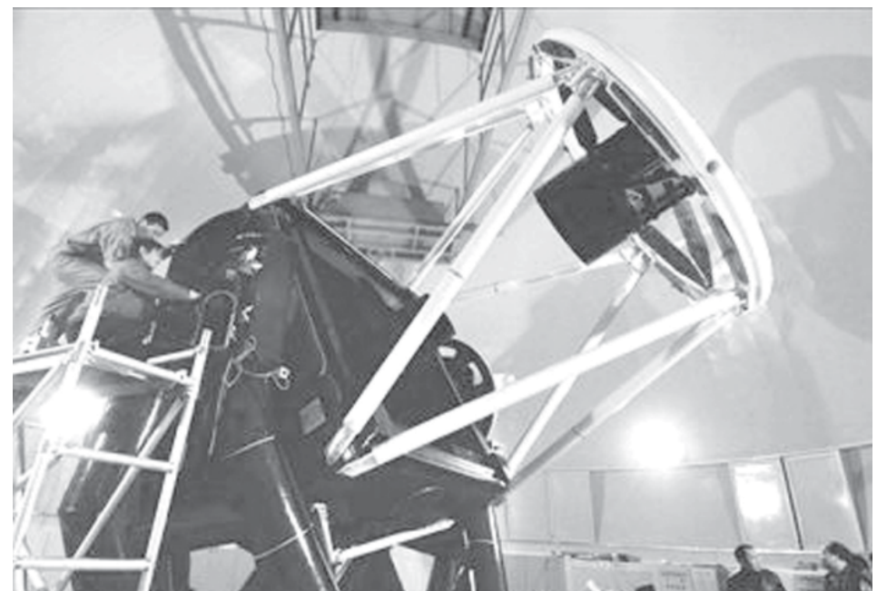
Technicians at Yunnan Observatory debug the optical telescope on 28 Jan, 2007. Asia’s largest optical telescope, with an aperture of 2.4 metres, a height of 8 metres and a weight of over 40 tons, has been installed at Lijiang Observation Station under Yunnan Observatory, the Chinese Academy of Sciences. —XINHUA
