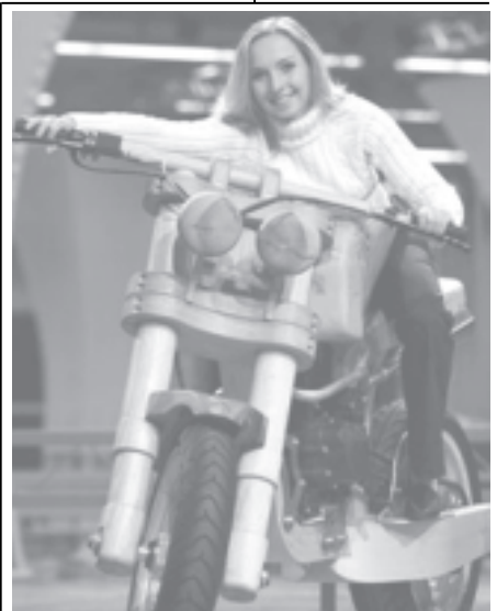
Model Marina poses on a motorcycle made of wood, which is powered by a 175 ccm/8 HP engine, and made by German joiner Michael Schoessler, during a Press presentation prior to the Essen Motor Show fair in Essen, Germany, on 21 Nov, 2005. —INTERNET
