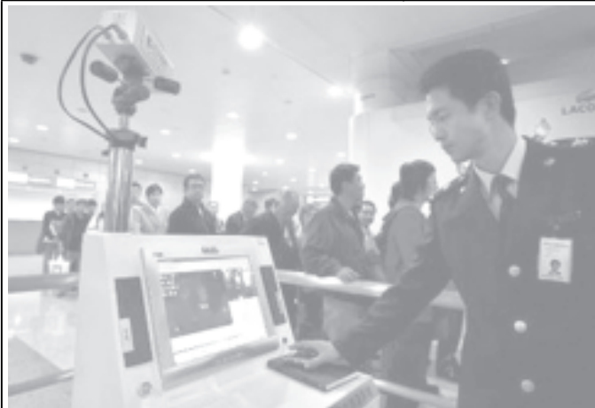
A Chinese airport security official uses a thermographic camera to check the body temperature of incoming passengers, to prevent people with fever entering, at Shanghai's Pudong International Airport on 24 Oct, 2005.
