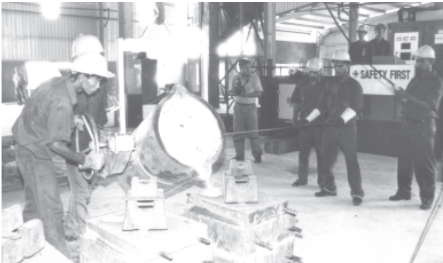
Workers casting iron at No 2 Foundry Plant of Modern Foundry Plant Project at Mandalay Industrial Zone.— MNA
