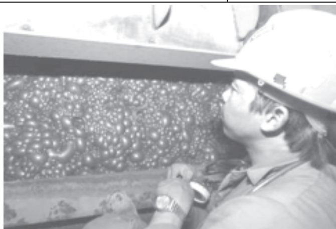
A Filipino mining engineer of Philex Mines observes the frothing process of high value minerals composed of gold, copper and silver at their milling plant in the northern Philippine province of Benguet on 28 Feb, 2005.—INTERNET
