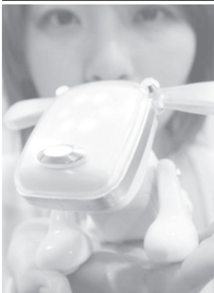
Eri Kameda, an employee of Sega Toys Co, Ltd with the toy maker's new pet dog robot, 'idog,' in Tokyo on 24 Jan, 2005. Depending on how the robot dog feels, 'idog' plays creative sounds. Owners can speak to it, sing for it, play music for it, and it communicates back with melodies. It can also dance if connected to a music player at a jack at its leg.—INTERNET
