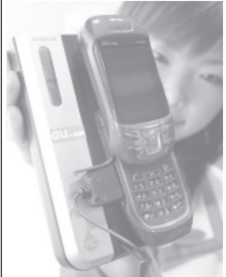
A model displays a prototype of a power supply for mobile phones using direct methanol fuel cell developed by Hitachi Ltd and au, KDDI's main mobile phone unit, at the International Fuel Cell Expo in Tokyo on 21 Jan, 2005.—INTERNET
