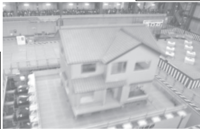
A group of invitees watch a two-storey model house being shaken by a huge amount of jolt created by a three-dimensional full-scale earthquake testing facility at Hyogo Quake-Resistance Research Centre, near Kobe, in western Japan, during its completion ceremony, on 15 Jan, 2005.—INTERNET
