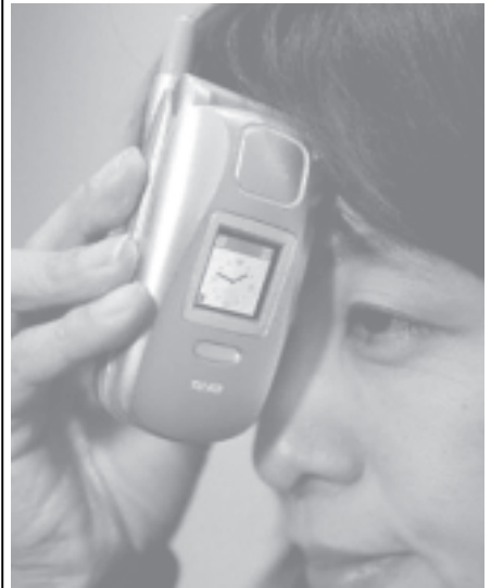
A Sanyo employee demonstrates Tu-Ka TS41 mobile phone, produced by Sanyo, which can transmit sounds with vibrations via the skull on 15 Jan, 2005. — INTERNET
