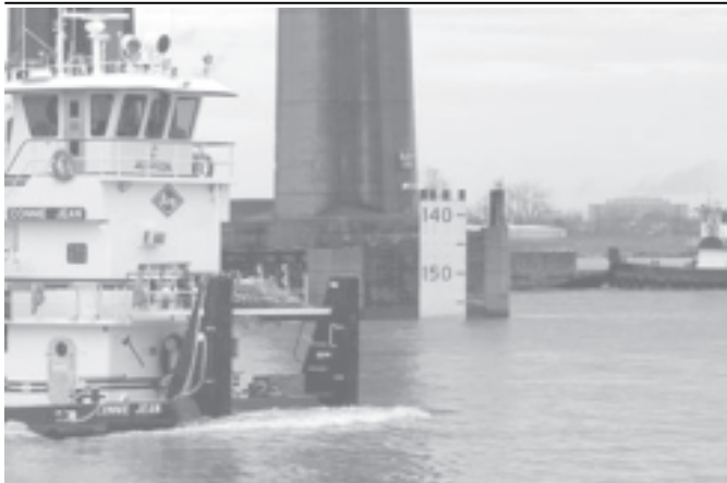
River traffic at the Crescent City Connection bridge which crosses the Mississippi River at New Orleans, approaches an air draft gauge that indicates the clearance from the river to the structure above, on 13 Jan, 2005. With the water running unusually high, large ocean-going vessels must keep a close eye on the clearance gauge.—INTERNET
