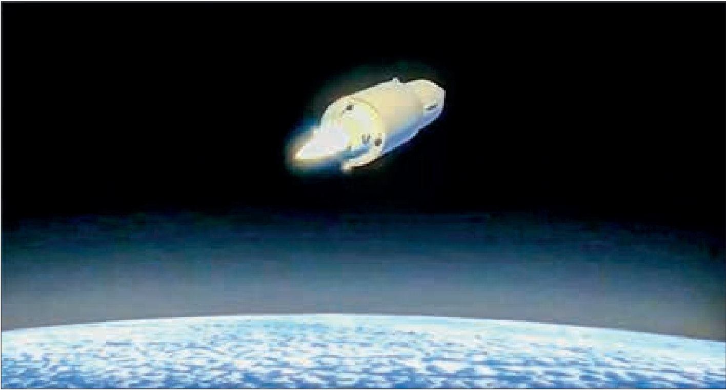
The Avangard is a Russian hypersonic glide vehicle (HGV) designed to be launched atop an intercontinental ballistic missile (ICBM). Unlike a conventional ballistic warhead, the Avangard can perform high-speed, sharp evasive manoeuvres as it glides towards its target.
