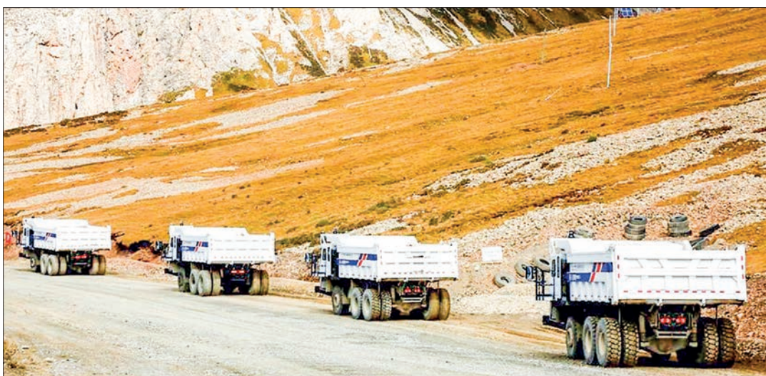
This undated handout photo shows hybrid autonomous trucks at the Yulong Copper Mine in Qamdo, southwest China's Xizang Autonomous Region. PHOTO: WESTERN MINING CO., LTD./HANDOUT VIA XINHUA
