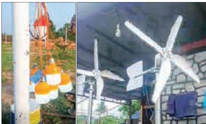
This image depicts a locally manufactured wind electric fan.
