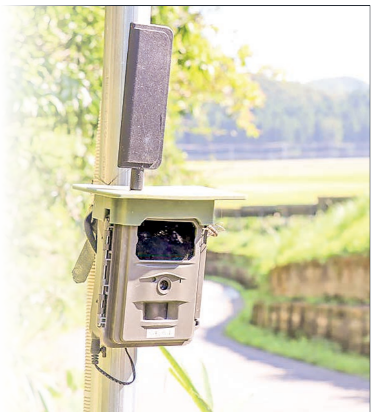
Photo taken on 6 September 2024, shows a camera installed in Komatsu, Ishikawa Prefecture, to monitor bears using an artificial-intelligence based system. PHOTO: KYODO
