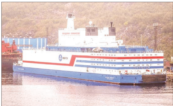
The Akademik Lomonosov is Russia's first floating nuclear power plant, designed to provide energy to remote areas and coastal regions. PHOTO: SPUTNIK
