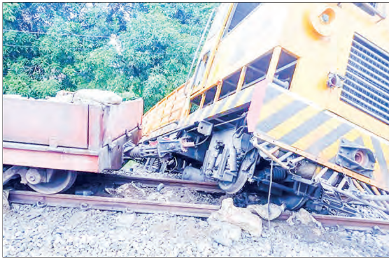
Photos (left & right) show The RGC 89 rail vehicle derailed after a mine blast.
