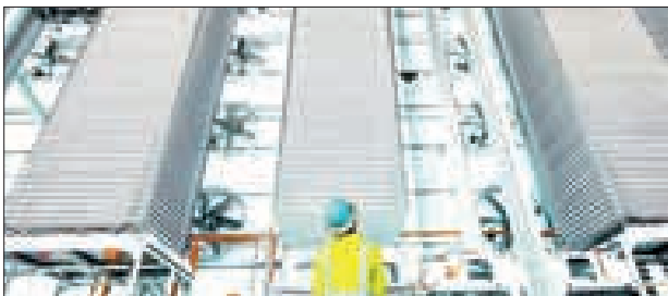
Heirloom's Direct Air Capture (DAC) facility in Tracy, CA uses limestone rocks to pull already-emitted CO2 from Earth's atmosphere. PHOTO: HEIRLOOM
