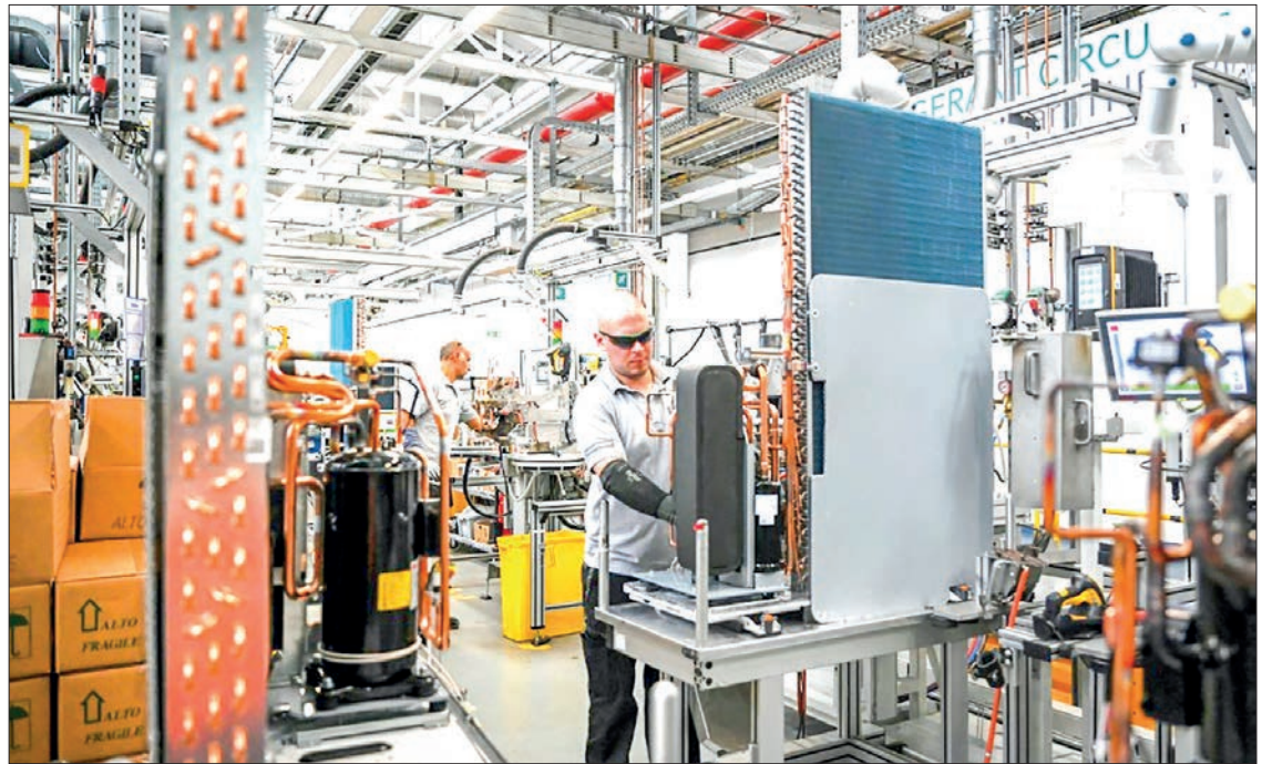
Employees manufacture the cooling unit for an air-to-water heat pump at the headquarters of the heating technology company Vaillant Group in Remscheid, Germany, on 20 July 2023. PHOTO: INA FASSBENDER/ AFP
