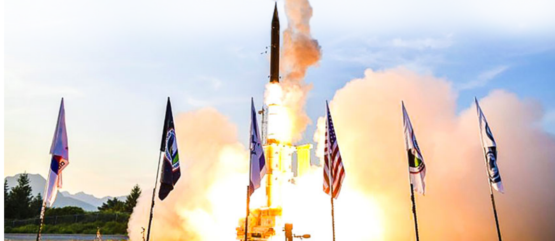
The Arrow 3 system — jointly developed and produced by Israel and the United States — is an interceptor designed to shoot down ballistic missiles above the atmosphere. PHOTO: ISRAELI MINISTRY OF DEFENCE/AFP
