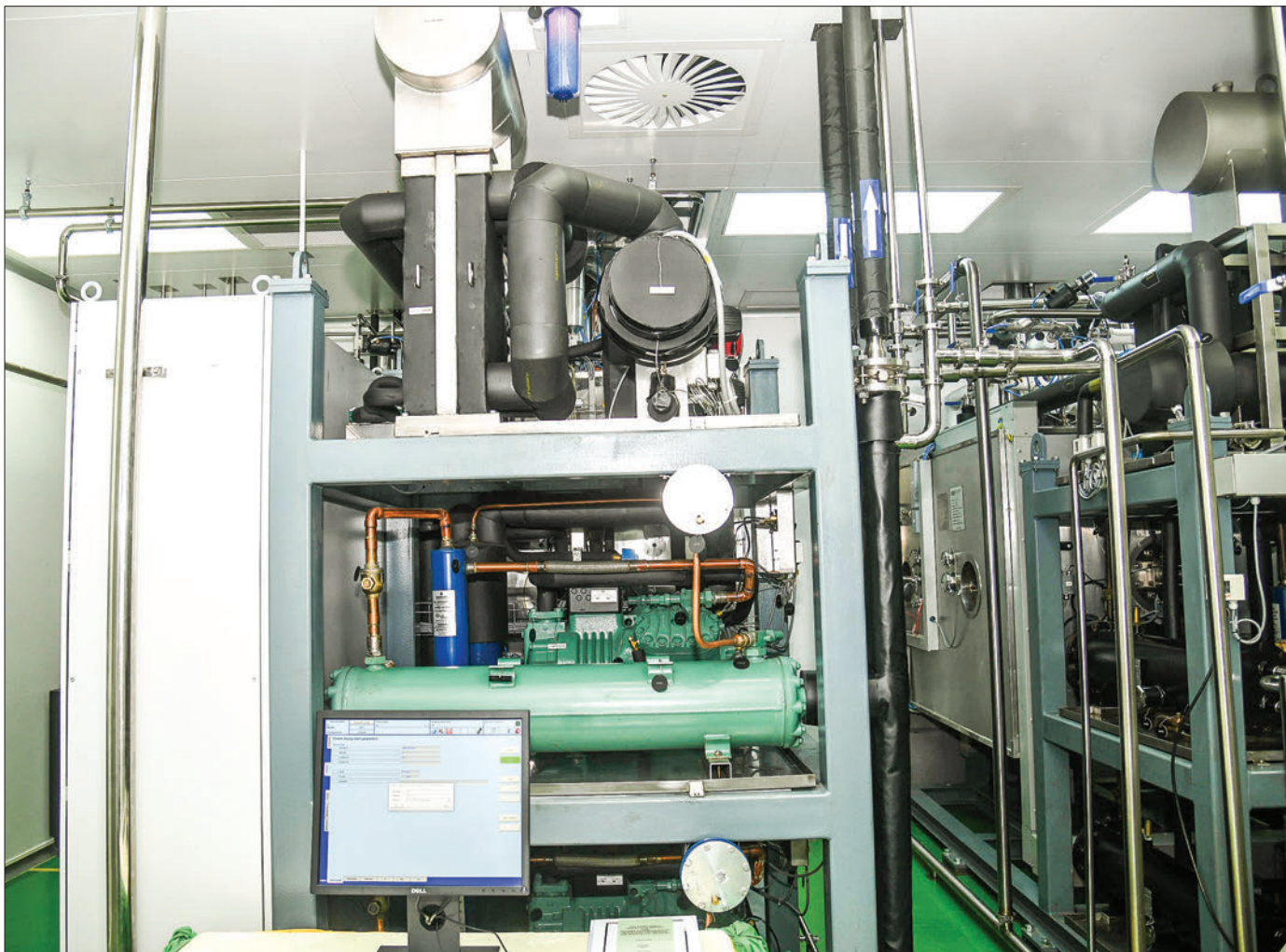
Cutting-edge freeze-dryer machine in operation for anti-snake venom production at State-owned BPI (Insein).
