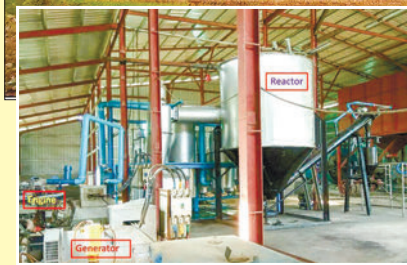
Homemade gasifier and its use for electricity generation (above and left photos.)
