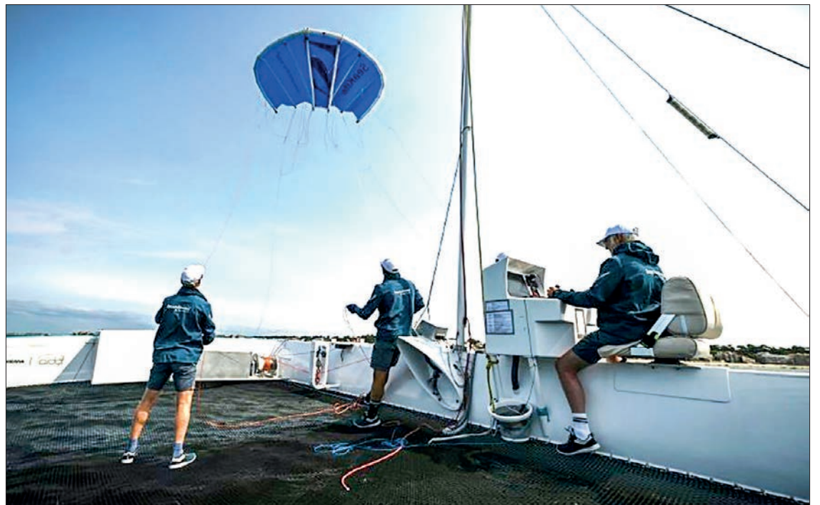
The startup Beyond The Sea tests a blue inflatable kite sail the size of a small studio to pull a specially-designed catamaran across the water. PHOTO: AFP/FILE
