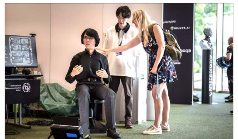
Visitors interacted with Geminoid HI-2, a tele-operated android created by Hiroshi Ishiguro Laboratories. PHOTO: FABRICE COFFRINI / AFP
