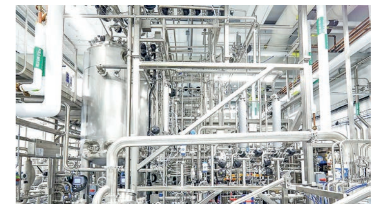
Some of the large cultivator tanks where meat is grown from meat cells, not from animal bodies. PHOTO: UPSIDE FOODS
