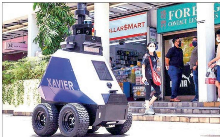
The robots are equipped with cameras, sensors, speakers, a display panel, blinkers and a siren. Singapore's Home Team Science and Technology Agency (HTX) roving robot has hit the streets of Toa Payoh Central as part of a trial to support public officers in enhancing public health and safety. **PHOTO: AFP/FILE**
