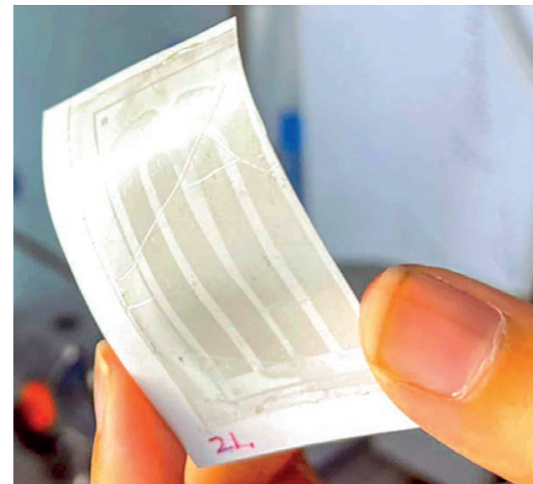
The implant is thin and flexible enough to conform to the heart's delicate contours as well as stretchy and strong enough to withstand the dynamic motions of a beating heart. Graphene tattoo patch. IMAGE CREDIT: NING LIU/UNIVERSITY OF TEXAS AT AUSTIN.
