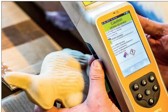
A Belgian customs officer at Brussels Airport using a Raman scanner to show that what appears to be a chocolate bunny is actually ecstasy. PHOTO: AFP
