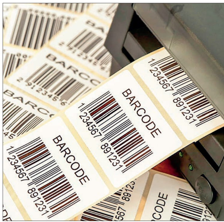
A barcode or bar code is a method of representing data in a visual, machine-readable form. Initially, barcodes represented data by varying the widths, spacings and sizes of parallel lines. PHOTO: AFP
