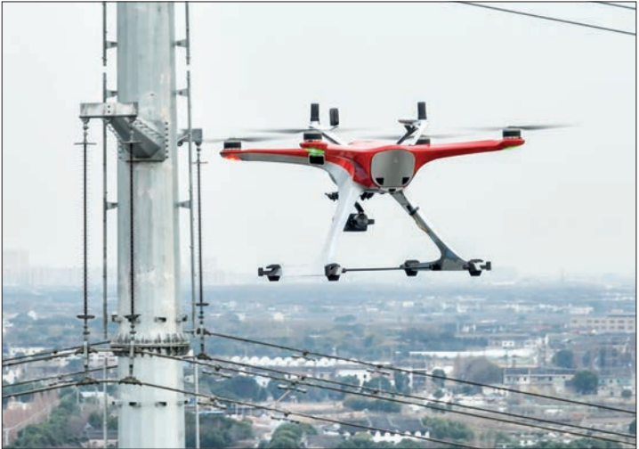
An unmanned drone with centimeter-level high-precision positioning capabilities inspects the automatic transmission lines of the electric transmission towers in east China’s Jiangsu Province, 29 Dec 2022. PHOTO: STATE GRID JIANGSU ELECTRIC POWER CO., LTD./ HANDOUT VIA XINHUA
