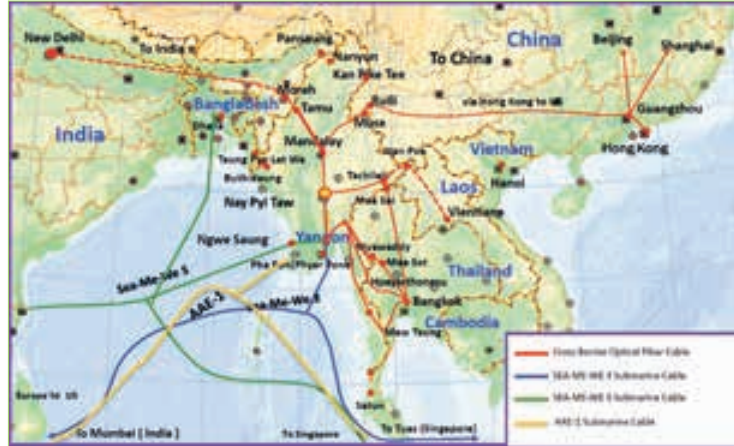
Submarine Cables and Cross Border Cables in Myanmar, Source: MOTC, Myanmar
