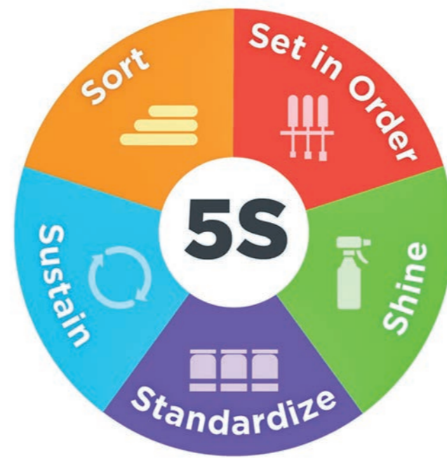
5S is a system for organizing spaces so work can be performed efficiently, effectively, and safely. IMAGE CREDIT: 5S TODAY
