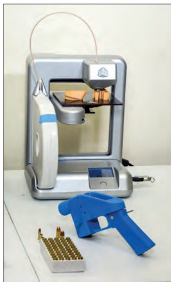
A Liberator pistol appears on 11 July 2013 next to the 3D printer on which its components were made. The single-shot handgun is the first firearm that can be made entirely with plastic components forged with a 3D printer and computer-aided design (CAD) files downloaded from the Internet. PHOTO: AFP / ROBERT MACPHERSON / FILE
