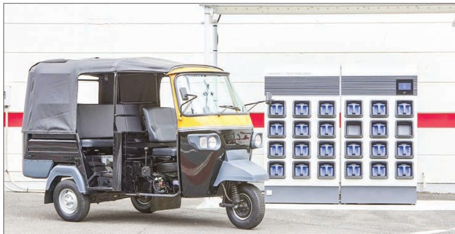
Supplied photo shows an electric tricycle taxi used in India parked in front of a station keeping Honda Motor Co.'s portable lithium-ion batteries. PHOTO: KYODO
