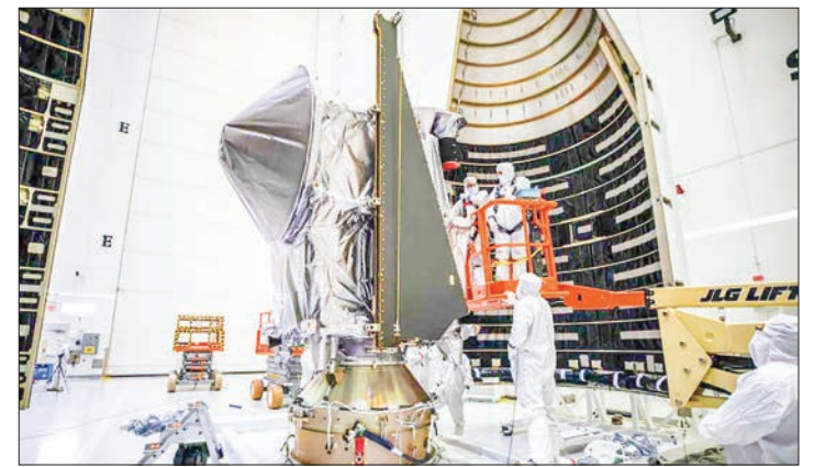
Workers inside the Astrotech Space Operations Facility in Titusville, Florida, move the first half of the United Launch Alliance (ULA) payload fairing toward NASA's Lucy spacecraft on 30 September 2021. PHOTO: NASA/BEN SMEGELSKY
