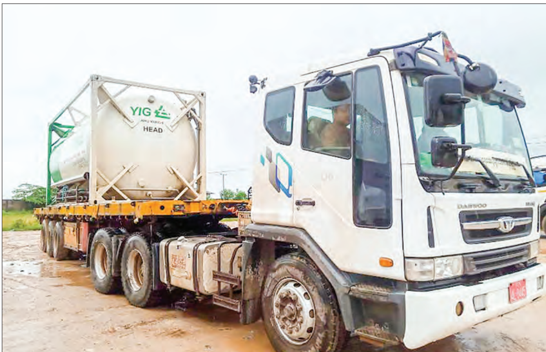
A truck is carrying liqued oxygen tank.
